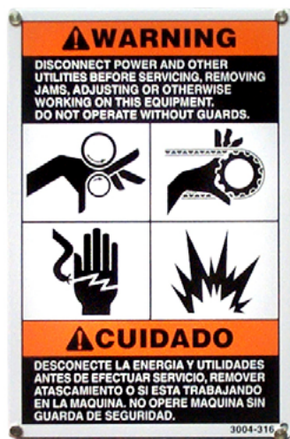
Figure 1-2: Safety labels remind operators and maintenance personnel that care must be taken when working near these areas.
