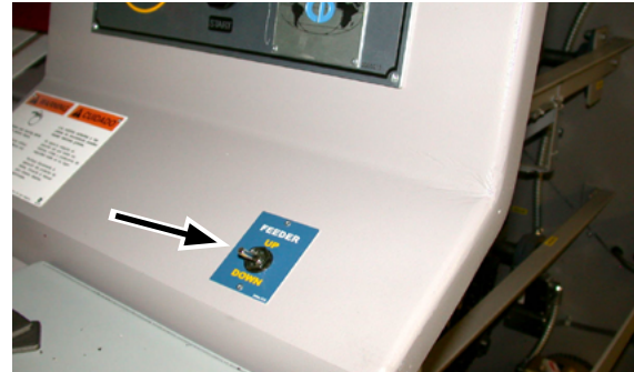
Figure 2-14: The O.P.L. UP/DOWN switch is located on the ironer's front endframe.
